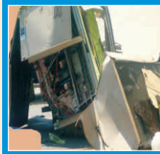
Locked Rotor Resulting in Burnt Compressor
