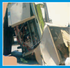
Locked Rotor Resulting in Burnt Compressor
